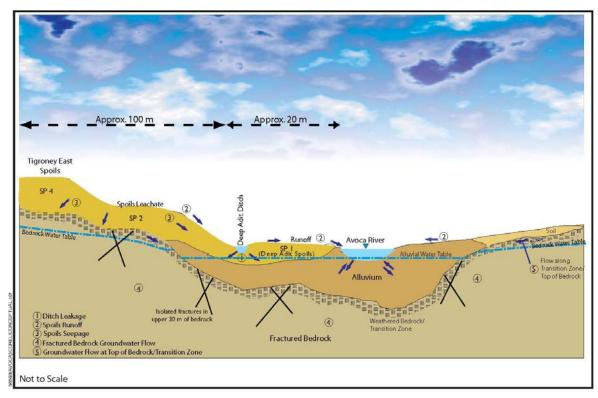
Figure 2-6 Schematic Cross-Section of the East Avoca Area Upgradient of the Deep Adit
