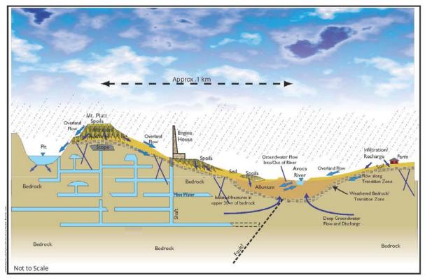
Figure 2-5 Schematic Cross-Section of Flow Components Influencing the Avoca River
