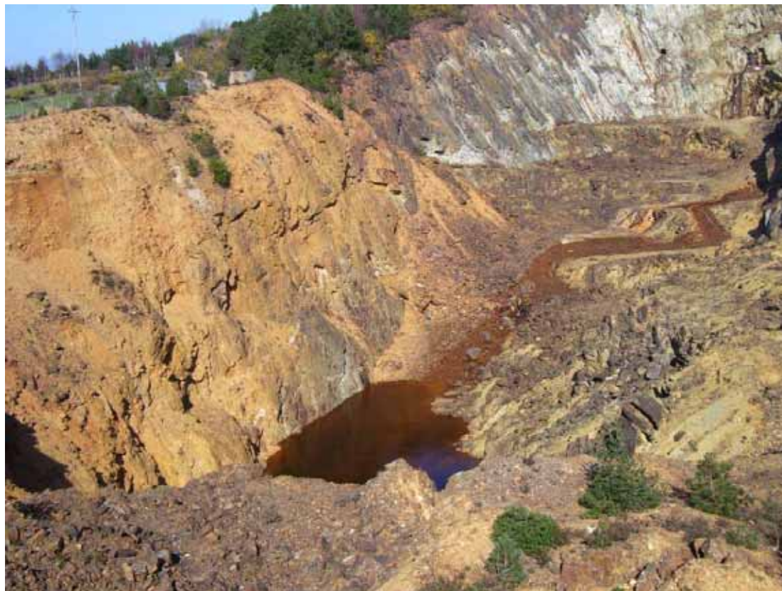
Figure 3-2 East Avoca Pit, showing the Intermediate Adit discharge flowing into the pit pond (April 2007).
