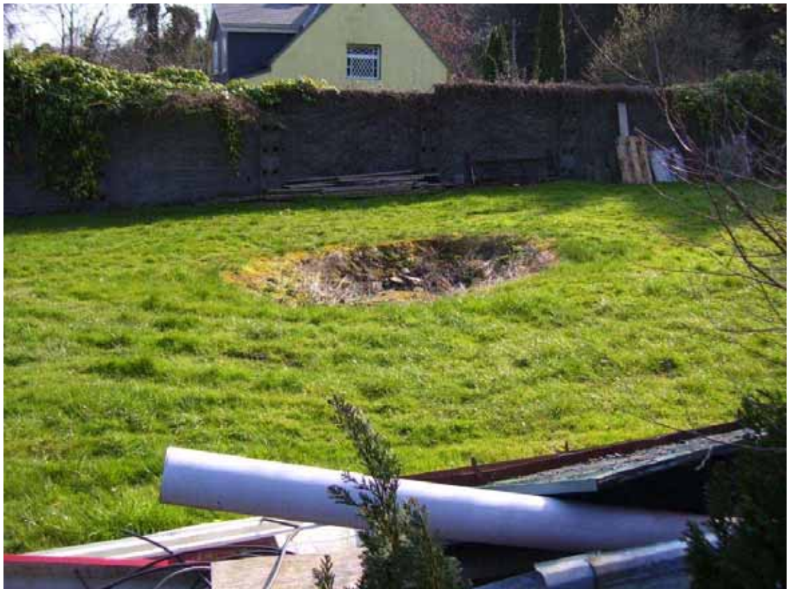
Figure 5-10 Sinkhole likely caused by prior subsurface discharge of the Ballygahan Adit.
