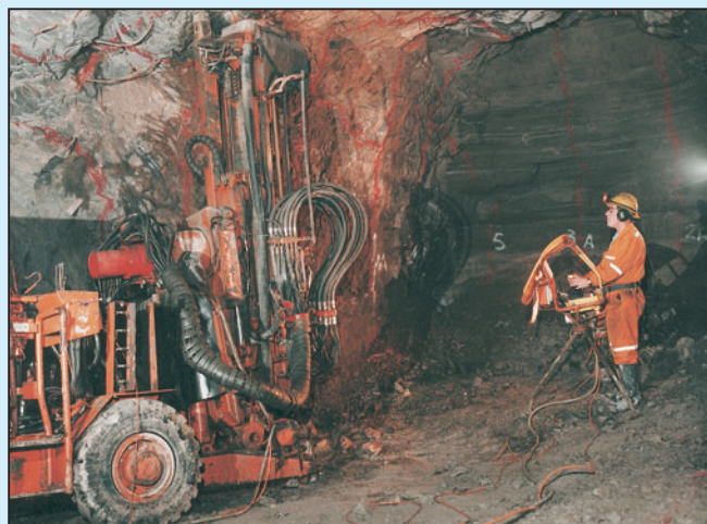
Underground Zn-Pb mining at Navan, Co. Meath (Courtesy: Tara Mines Ltd.).
