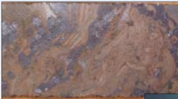
Brecciated banded sphalerite invaded by coarse-grained galena. Assay 30.15% Zn, 41.29% Pb, 178 g/t Ag. Core at 155.3m depth from the R Zone, Galmoy deposit. (Courtesy Arcon Exploration Plc)
