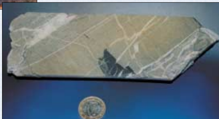
Core from Tullybuck-Lisglassan gold prospect, grading 32 g/t Au. (Courtesy Conroy Diamonds and Gold Plc)
