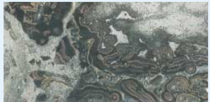
Galmoy rock matrix breccia (x 3) showing sphalerite and galena. (Courtesy: Irish Association for Economic Geology).
