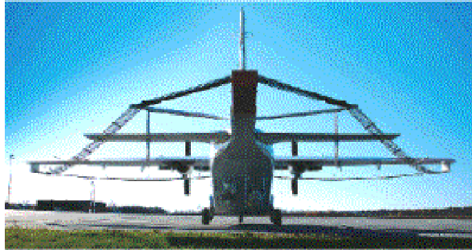
Figure 1: View from the rear of a Fugro survey aircraft (Shortt's Skyvan), which can simultaneously acquire magnetic, radiometric and time domain electromagnetic data.
